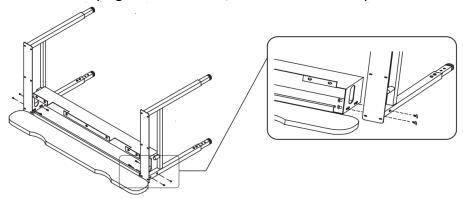
**Step 2:** Place the table top on a smooth, clean surface with the bottom facing up. Align the assembly from step one with the predrilled holes in the larger top. Verify the alignment before moving to step 3.
