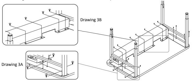
**Step 4:** Adjust the PSD leg inserts to the desired height and secure with (8) 3/8-16X.625 half dog nut screws (2 per leg). Use the provided allen wrench to loosen and tighten the screws.
