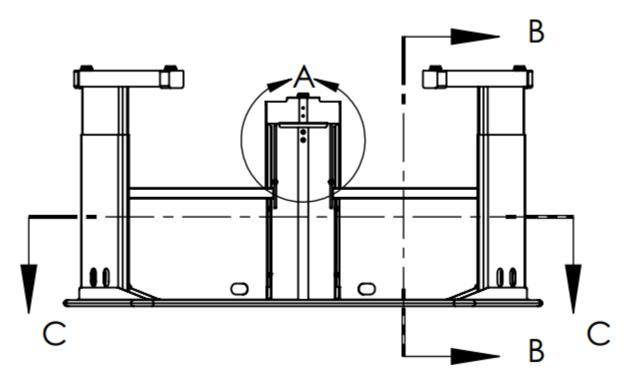
Step 1: On a clean flat surface, flip the top upside down so that the pre-drilled holes are visible. As shown in figure 1, attach the two modesty panels to the center leg using the large 1/4-20 machine screws (2 per panel). Do not tighten completely.
