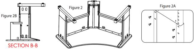
Step 3: With the legs and the panels assembled loosely, align them with the pre-drilled holes and attach them to the top with the supplied wood screws. Now tighten the machine screws between the legs and the panels.
