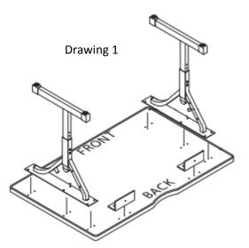
**Step 3:** Loosely attach the Panel to the Y-Legs using the (4) Connector Bolts (See Picture #2). ONLY HAND TIGHTEN THE BOLTS.
