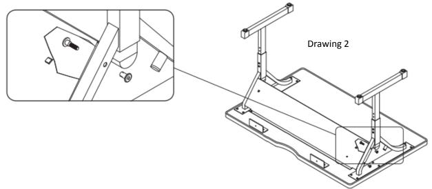
**Step 4:** Using the remaining wood screws, attach the Y-Legs and the panel to the top. Go back and tighten the bolts from Step 3.
