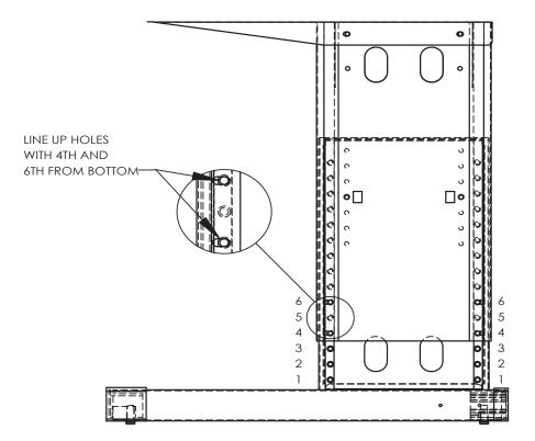
Step 2A (If you cabinet is a Box Box File): Place the Box Box File (BBF) upside down on the table top opposite the leg. Align the modesty panel with the two holes on the BBF and the leg. Attach the modesty panel to the BBF and the leg using (4) 1/4-20 machine screws. The screw holes on the BBF are along the outside of the top plate (as seen inthe picture).
