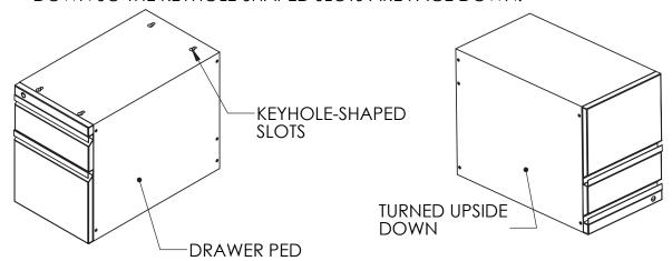
3. SECURE DRAWER PED ON MOUNTING PLATE. ALIGN SLOTS ON DRAWER PED TO KNOBS ON MOUNTING PLATE. BE CAREFUL NOT TO FORCE THE PARTS TOGETHER. THE KNOBS ON THE PLATE SHOULD COMFORTABLY ALIGN WITH THE SLOTS. ONCE THE PED IS SEATED ON THE PLATE, SLIDE THE PED FORWARD (TOWARDS YOU).
