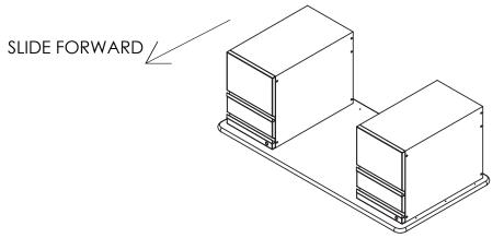
5. ATTACH LEGS TO DRAWER PEDS USING CONNECTOR BOLTS
