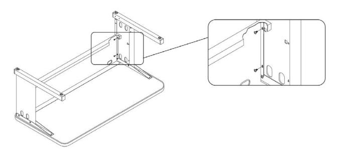
**STEP 4:** Attach the cross brace to the foot using the (4) 10 - 32 x 1/2" machine screws.
