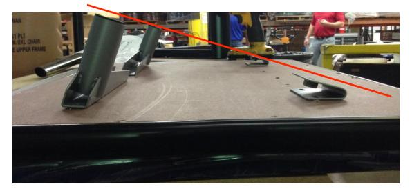
**Step 2:** Attach the Lectern Poles and the brackets to the top using the provided wood screws. Notice that the arrows on the brackets point toward the INTERIOR of the top once in position.
