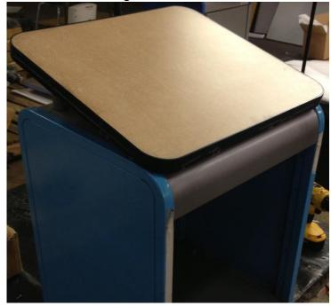
**Step 4:** Attach the Top to the cascade unit by using the 1.25" bolts on the rear with the poles, and the 0.5" bolts on the front with the brackets. Be sure to use the washers on the inside of the unit, when attaching the bolts from underneath.
