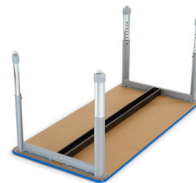
24", 30" & 36" deep activity tables feature one center support channel 2" x 3" wide 14-gauge steel, with 11-gauge steel endplates for stability
