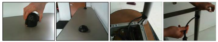
Step 6: Using attached cable ties, neatly tie up the cables in bundles under the table.
