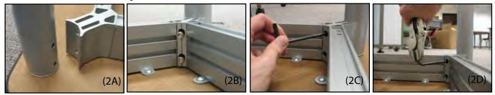
Step 3: Place the Leg Stabilizers (Wall or Island) onto the bottom of the UXL legs and use the M8x25 countersunk screws provided to fasten the stabilizers to the legs.
