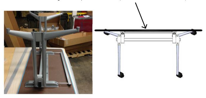
Step 5: Attach both legs to each side of the beam and tighten using a 5mm Allen Wrench, bolts, and plate removed in Step 2.
