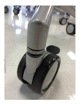
Step 8: To level table, adjust caster up or down by turning the hex nut below silver knurled disc - clockwise or counter-clockwise until level. Lock in place by turning.
