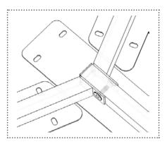
after the frame assembly is secured to the top, completely tighten the connector bolt with the Allen Key provided.
