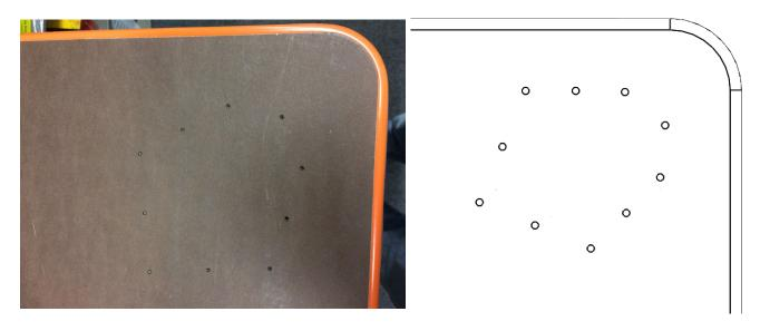
Step 2: Align table leg with pattern and install 10 screws. Repeat for each leg.
