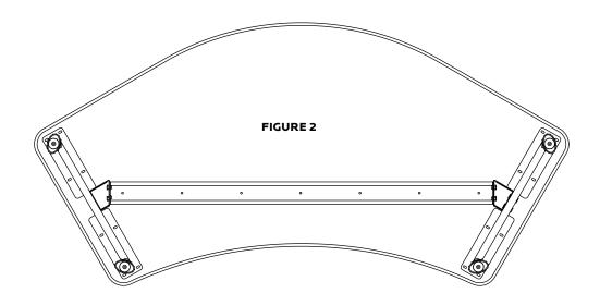
\*tip\* stagger screws during assembly; i.e. fasten one screw into one of the legs, then another screw on the other leg. Continue to stagger until all screws are used.
