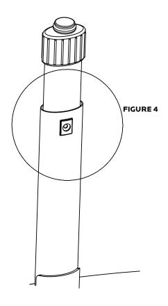
**STEP 6:** Adjust the leg height as desired by loosening the set screw in each leg (using the Allen Key provided). Move leg to desired height - and be sure to locate the appropriate hole in the leg.
