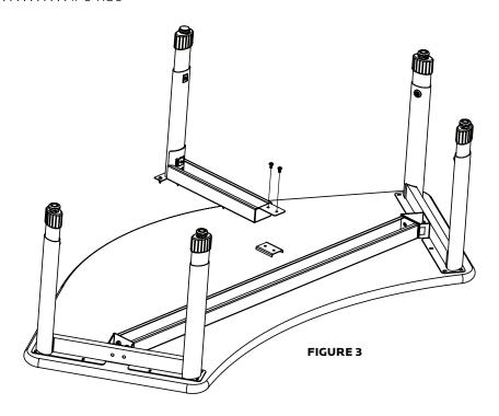
STEP 5: Rotate the T-Nut bracket 90° and insert into channel support. Loosely attach 1 / 4-20 screws through the single leg bracket (#26663). Maneuver single leg bracket until screw holes align with predrilled holes in the top - Install Screws.
