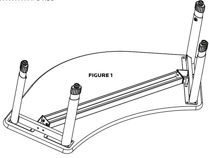
**STEP 1:** Place the top on a clean,dry surface laminate side down, so that the predrill holes face up.
