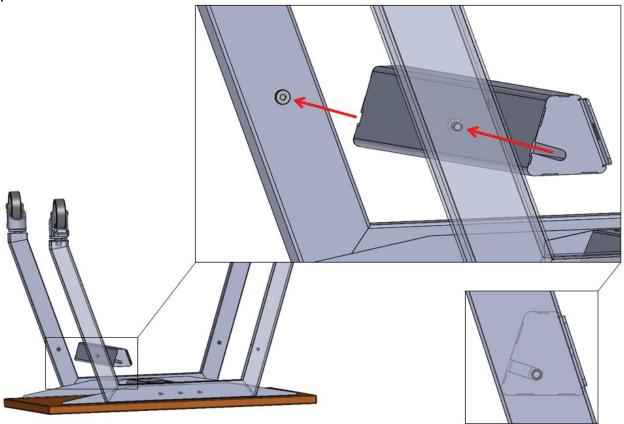
5. Secure rails into place by installing the 1/4-20 Pan Head Screws as shown.
