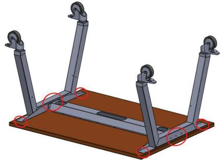
3. Using a 3/16" allen wrench, install 1/4-20 Shoulder Bolts as shown on all 4 legs.
