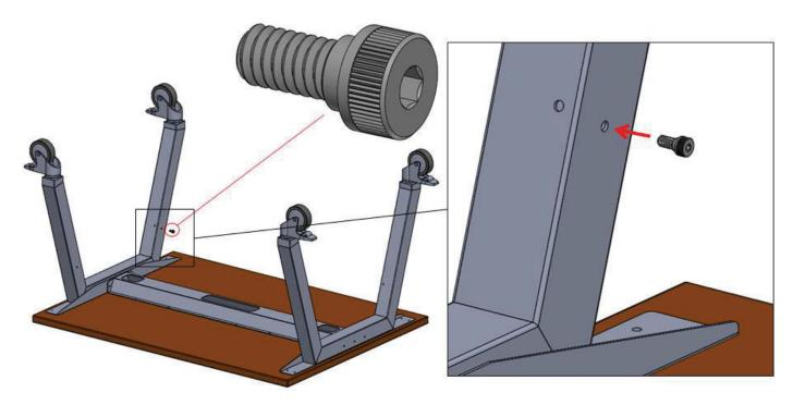
4. With a partner, install rails by aligning slots on rail ends with shoulder bolts and sliding rails into position as shown.
