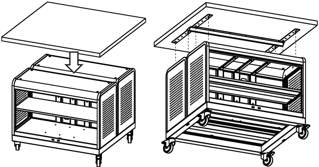
6. Attach the top to the cases using the 3/8" x 1 1/4" OD oversized washers and 3/8"-16 lock nuts with a 9/16" socket & ratchet, or 9/16" wrench.
