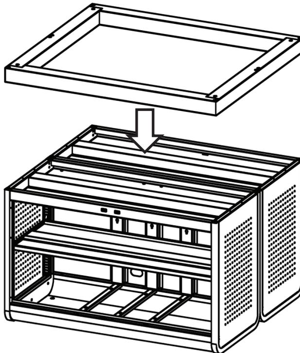
3. Attach the base to the cases using the 3/8"-16 x 3.5" bolts and 3/8" lock washers.
