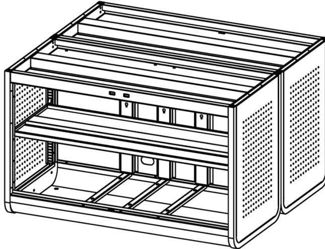
2. Position the base onto the cases and line up holes, as shown. **Base is heavy, team lifting is advised.**
