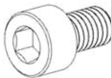
M6 X 1.0MM X 10MM SOCKET HEAD BOLT (PN: 60059) QTY. 8
