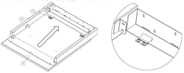
6. Install items #5 and #4 to item #3 as shown using 4x fastener item #3, finger tighten only.
