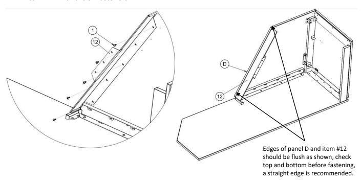
11. Align item #9's edge with the reference line as shown. Item #10 can be used as a spacer for panel C. Insert panel C into the slot of Item #12. Place item #9 against panel C as show. Confirm that all 3x holes on item #12 and item #9 can be seen though the slots while item #10 is in place. Fasten #12 and #9 to panel C using 3x fastener #1 each. (Do not fasten item #9 to the panel H, this will be done in
