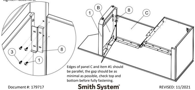
13. Edge of item #1 should be parallel with the reference line as shown (depending on the assembly process the reference line may not be flush with the edge of item #1) Align edge of tube from item #1 with the edge of the wood, NOT the face of the edge banding. Fasten #1 to panel H using 8x fastener #1 and then faster item #9 to panel H using 3x fastener #1.
