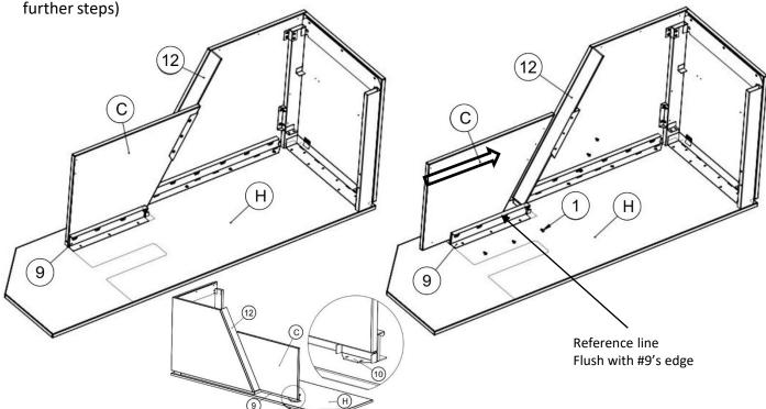
12. Place the previously assembled item #1 and panel B as shown. Attach item #8 using 2x fastener #1 to panel C and attached item #8 to item #1 using 2x fastener #3, finger tighten only. Confirm the gap between item #1 and panel C is constant and as minimal as possible as shown below. Fully tighten fasteners.
