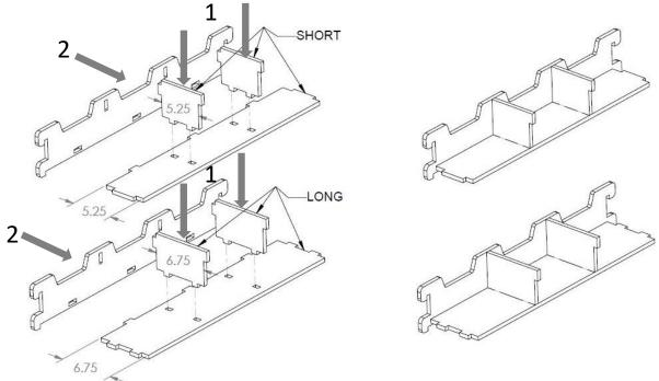
3. Lay "Front Panel" on a flat clean surface. Align the mating geometry as shown, the parts should mate without gaps.
