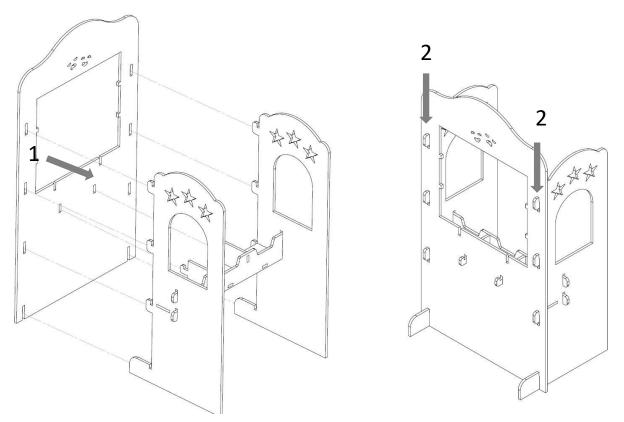
6. Carefully align the side panels with all mating nubs. The side panel should slide over the hooks first then the nubs. An extra set of hands helps, do not force the parts. A gentle tap with the palm of your hand is sufficient to seat the parts.
