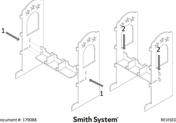
5. Carefully align the front panel with the previously assembled panels, slide the panel over the hooks then slide the front face down to lock the hooks into place.
