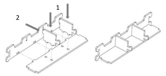
3. Carefully align the side panels with all mating nubs. The side panel should slide over the hooks first then the nubs. An extra set of hands helps, do not force the parts. A gentle tap with the palm of your hand is sufficient to seat the parts.
