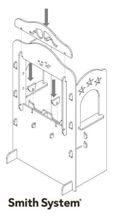
10. Align the mating geometry as shown, slide the display frame over the hooks then slide down to lock the display frame into place.
