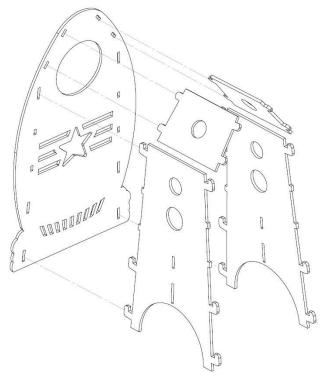
3. Align the mating geometry as shown, the parts should mate without gaps.
