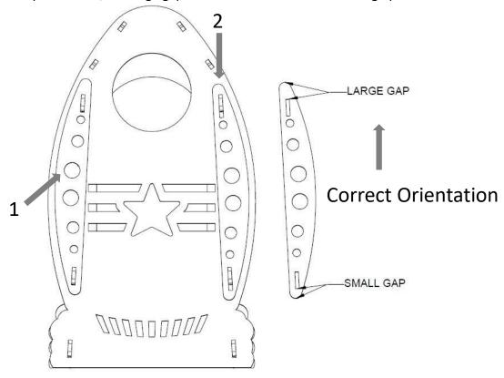
5. Install the lower connectors by pushing over the nubs then pushdown to lock the connector in
